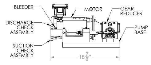
Model A & Model B electric pumps are designed for continuous and intermittent pumping of chemical and corrosive fluids.
